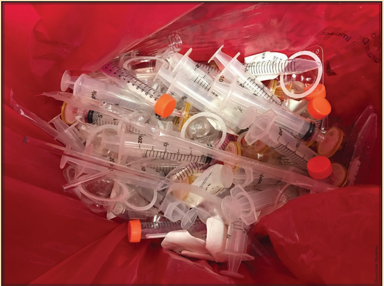
In an HIV testing laboratory, single-use plastic syringes, pipettes, and filters are disposed of in a red hazardous materials waste bag.
