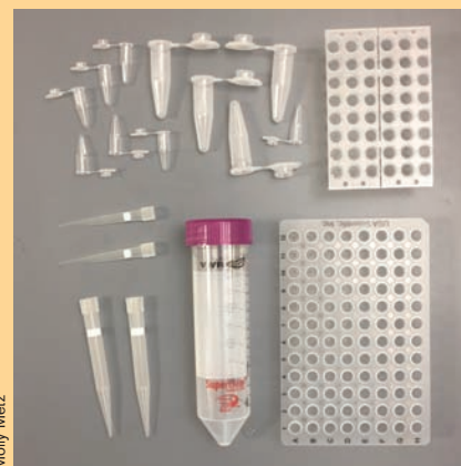
Figure 2. Commonly used, single-use plastics or “consumables” from the laboratory. A selection of conical tubes, PCR tubes, filter tips, multi-well plates and microcentrifuge tubes are shown.
